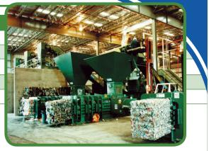
enclosures for workers; and storage cages for sorted materials with automatic discharge to the baler feed conveyor.
